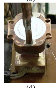
Figure 2: Components of MSRS for electronics cooling: (a) Reciprocating compressor; (b) Microchannel condenser; (c) Needle valve and capillary tube; (d) Microchannel evaporator-copper heater block.
