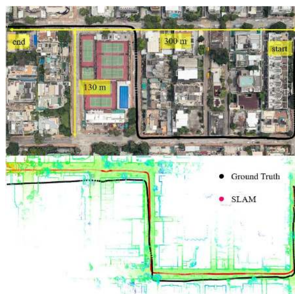
Figure 8. Experiment 2: the trajectory of NDT-based graph SLAM in a sparse area with dense traffic condition. Top panel represents the snapshot in Google Maps. The black curve indicates the ground truth of the vehicle's trajectory. The bottom panel indicates the generated points map and trajectory from SLAM.
