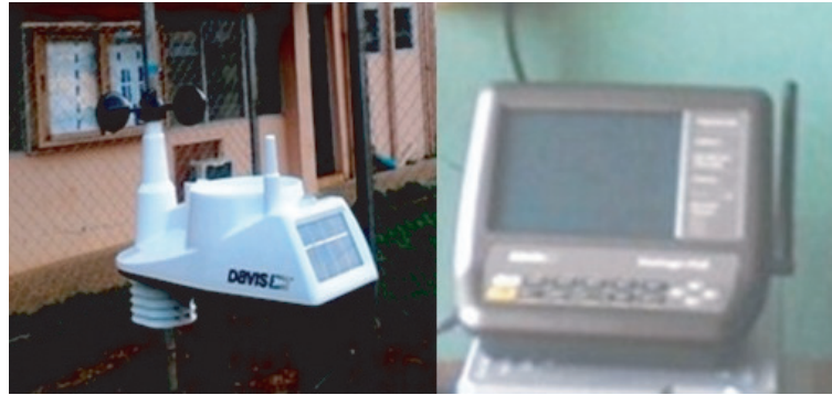
Figure 1. The outdoor ISS and the indoor console units of the Davis Vantage Vue electronic weather station.
