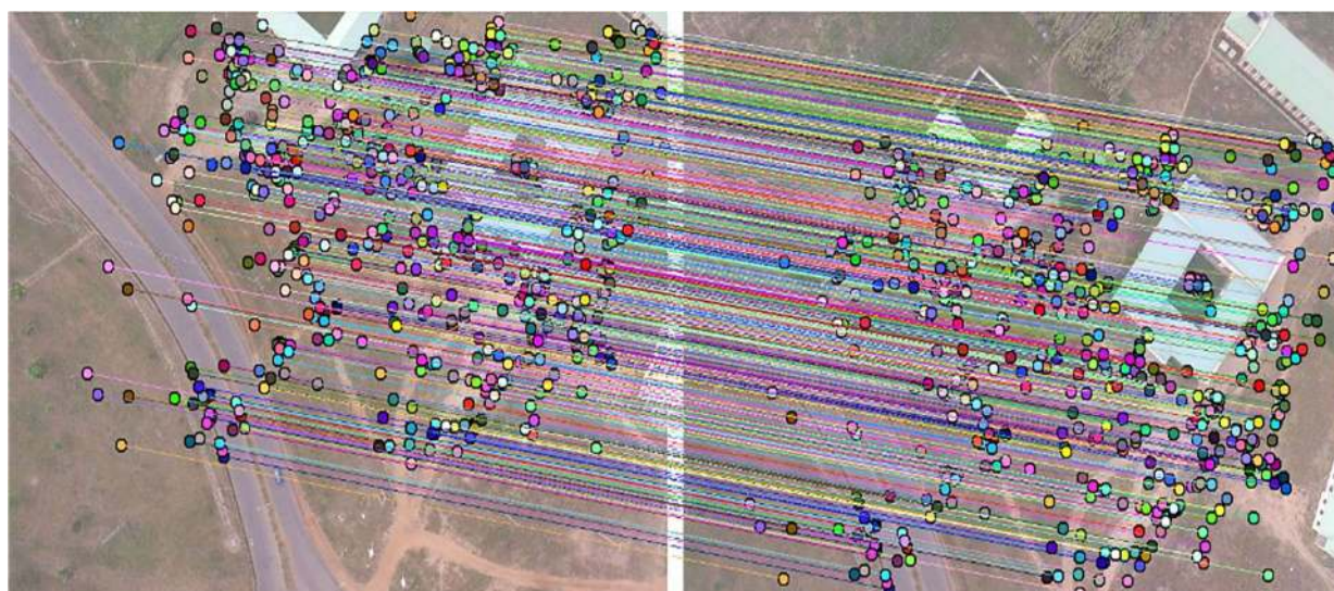
Figure 5b: Matched inliers using Speeded Up Robust Features Algorithm (SURF)
