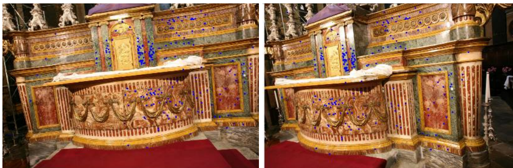
Figure 3. The Misericordia test. The image correspondences automatically matched with SIFT (303 points, Th_{eu} = 2 , L = 10 ).
