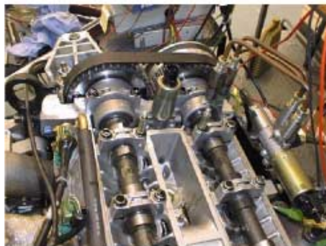
Figure 3 Ford 1.7L Zetec Engine with dual VCTs
