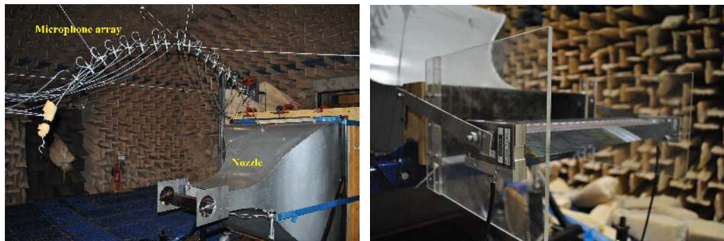
(a) Photograph of jet nozzle and test setup inside the ISVR anechoic chamber. (b) Photograph of aerodynamic measurements in an open jet wind tunnel.
