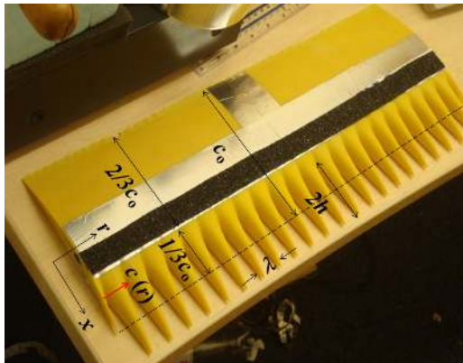
(a) Schematic representation of serrated leading edge (b) A photograph of the LE serrated aerofoil showing all the parameters
