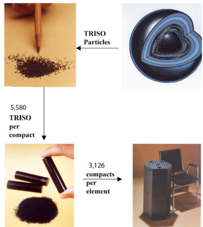
Fig. 3. TRISO particles, fuel compacts, and hexagonal fuel element.
