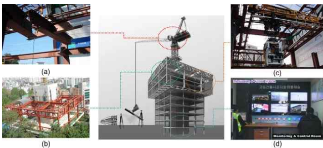
Figure 1. Structure of RCA system
