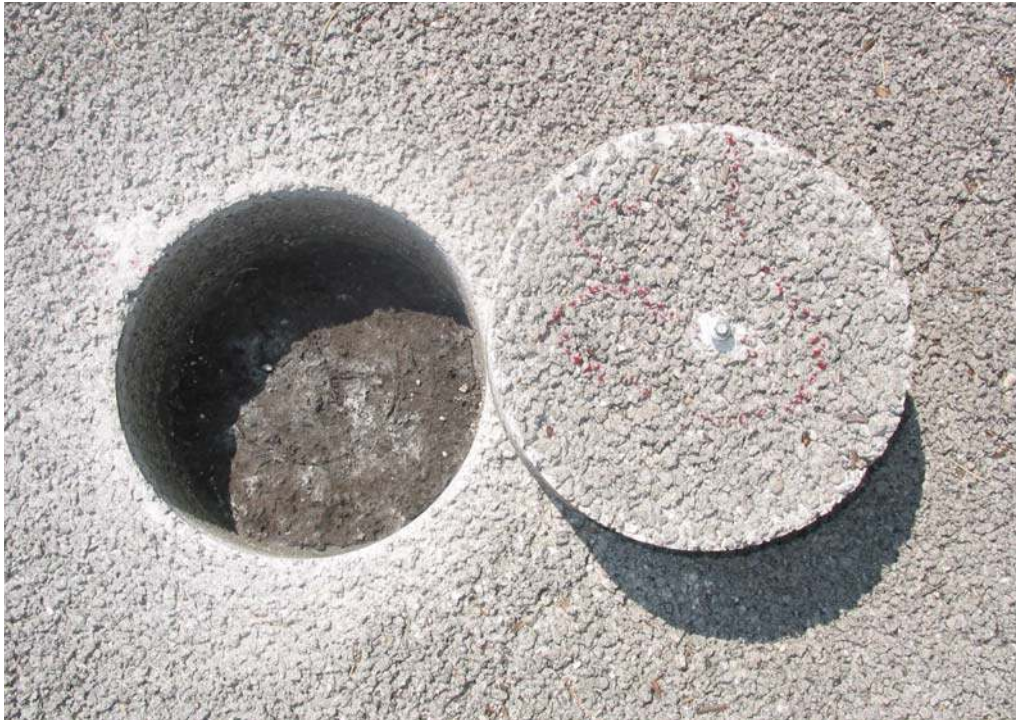
Figure 8: Pervious Concrete Pavement Core
