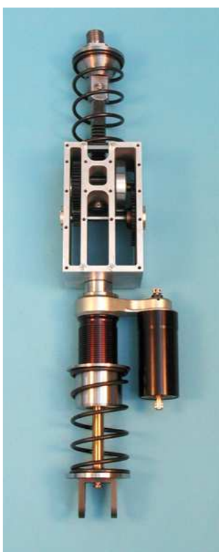
Figure 13: Inerter in series with damper with centring springs
