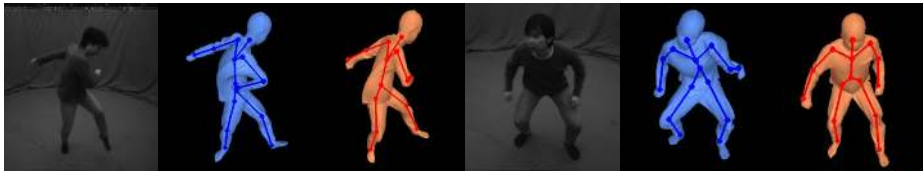
Fig. 4. Comparison with multi-view video tracking (MVT) approach on the “Jump” sequence. The left three and the right three are: input image, result of MVT, result of our Kinect-based approach. On this fast motion Kinect-based tracking succeeds while MVT fails to capture the arm motion.
