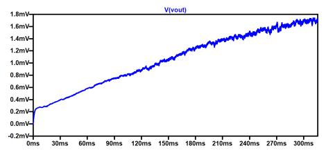
Figure 18. The output-voltage response of the circuit with Si-MOSFET-based switch and RLC Load.
