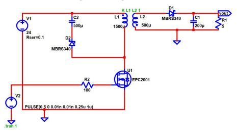
**Figure 10.** DC-to-DC flyback converter with resistive load of 5  $\Omega$ .
