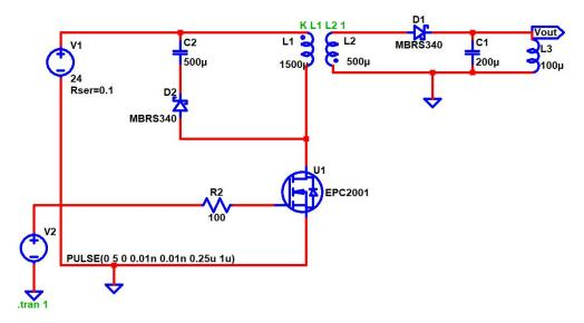
Figure 13. DC-to-DC flyback converter with inductive load configuration.
