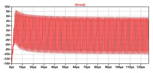
Figure 8. The output voltage response of circuit with GaN switch and resistive load configuration.
