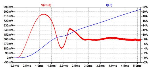
Figure 14. The output voltage and current response of the circuit with GaN switch and LC load.
