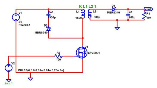
Figure 7. DC-to-DC flyback converter circuit response with a resistive load.
