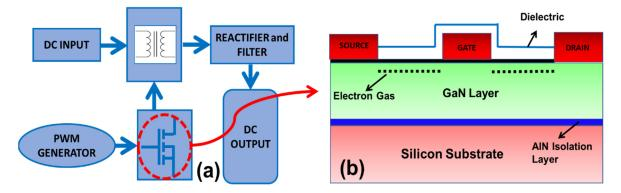
**Figure 2.** (a) Block diagram of flyback topology with PWM as input to the switch; (b) the internal structure of a GaN FET.
