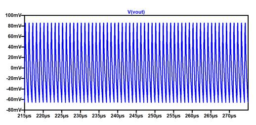
**Figure 9.** The output voltage response of circuit with Si MOSFET as switch and resistive load configuration.
