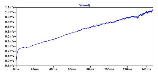
Figure 12. The output-voltage response of the circuit with Si MOSFET as switch and RC load at output.
