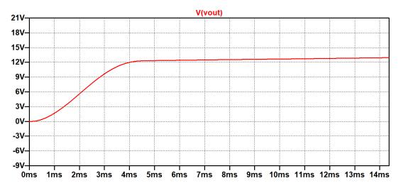
Figure 5. The output voltage response of GaN-FET-based switch for an open-circuit configuration.
