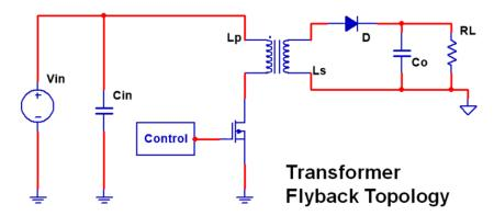
Figure 1. DC-to-DC converter with flyback topology.
