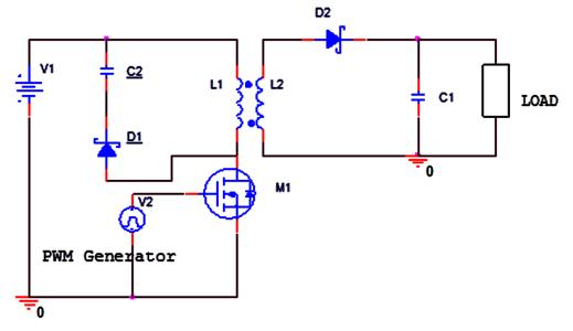
**Figure 3.** GaN-based active-clamp flyback converter topology with DC source, PWM generator, and load at the output.
