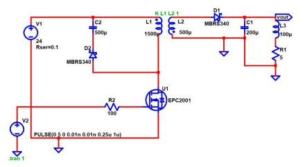
Figure 16. GaN-switch-based DC-to-DC flyback converter with RLC load configuration.
