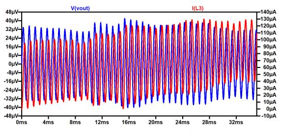
**Figure 15.** The output voltage and current response of the circuit with Si-MOSFET-based switch and LC load.
