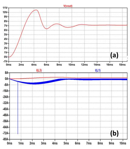
**Figure 17.** (**a**) The output voltage response with GaN switch and RLC load; (**b**) the input and output current responses with GaN switch and RLC load.
