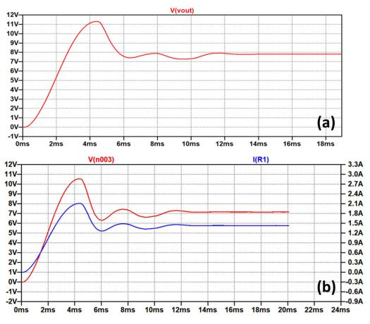
**Figure 11.** (**a**) The output-voltage response with resistive load; (**b**) the output current and voltage response of the circuit with resistive load.
