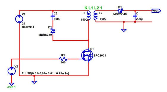
Figure 4. Open-circuit configuration of active flyback DC-to-DC converter.
