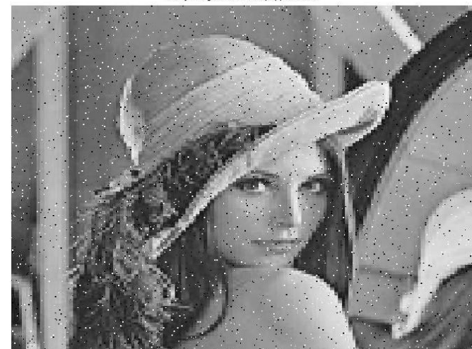
noisy image with salt & pepper noise Fig.3 Noisy image: Salt and pepper noise with noise density = 0.02
