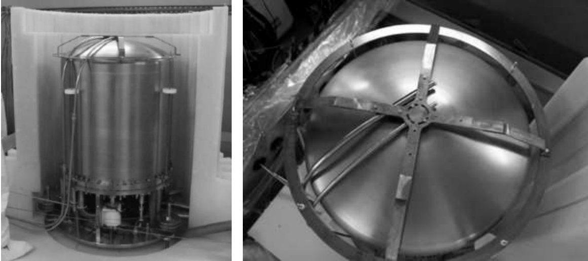
Figure 2. Left: ZEPLIN-III partially surrounded by the polypropylene slabs of the veto system. Two pipes of the source delivery system are attached to the vacuum dome. The detector leveling system with pulley wheels and cables can be seen at the bottom of the detector. Right: ZEPLIN-III viewed from the top. The gamma source was delivered through the pipe above the center of the detector, while the neutron source was placed on the top 5 centimeters off-centre.
