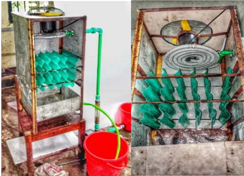
Fig. 6. Cooling tower with regular-shaped film fills
