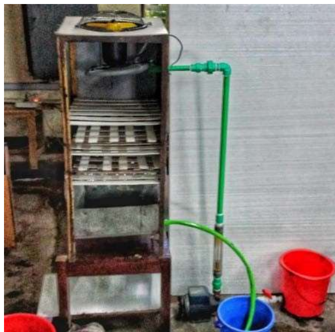
Fig. 5. Cooling tower with regular-shaped splash fills
