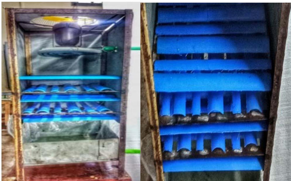
Fig. 7. Cooling tower with inverted u-shaped splash fills
