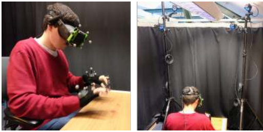
Figure 1: User shown typing in mid-air with HMD, hand and fingertip tracking markers (left). OptiTrack camera setup for precision marker tracking (right).
