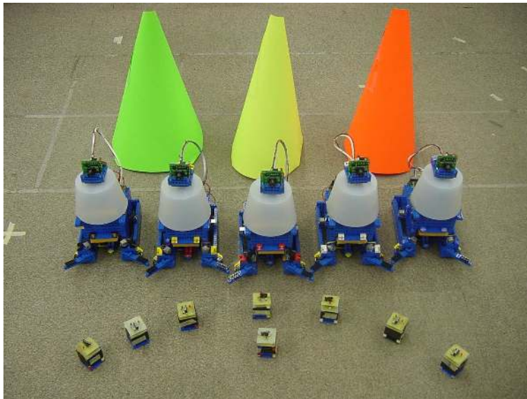
Figure 1: The Minnesota Distributed Autonomous Robotics Team (MinDART) with the infrared targets in front and colored landmarks in back. The MinDART robots searched for the infrared emitting targets in a search and retrieval task. Landmarks were used for homing and localization.
