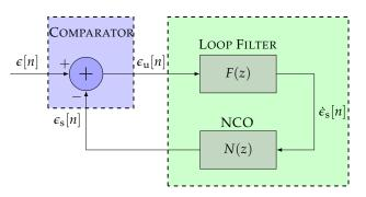
Figure 2. Linear model of the scalar tracking loop (STL).
