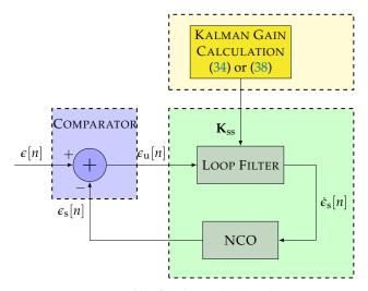
Figure 7. Linear model of lookup table (LUT)-DSKF.
