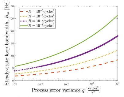
**Figure 6.** Relation between steady-state loop bandwidth  $B_{ss}$  and process error variance *q* in a third-order DSKF. ©IEEE. Adapted, with permission, from [20].
