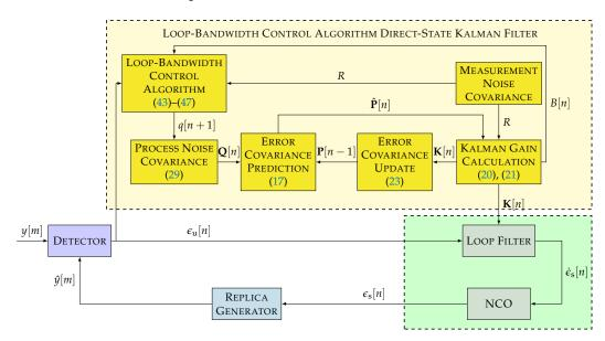
**Figure 9.** Non-linear model of loop-bandwidth control algorithm (LBCA)-based DSKF. ©IEEE. Adapted, with permission, from [20].
