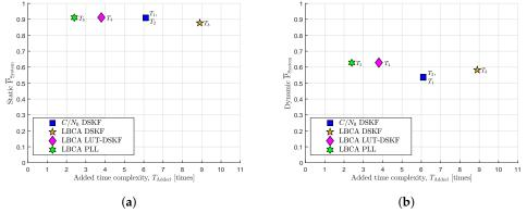
**Figure 16.** System performance vs. added time complexity comparison. (**a**) Static scenario. (**b**) Dynamic scenario.
