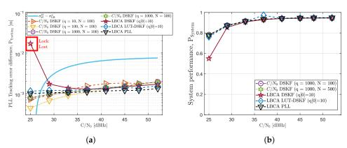
**Figure 14.** Static performance of adaptive tracking techniques in third-order Costas phase locked loop (PLL) at different  $C/N_0$  levels. (a) Tracking performance of satellite vehicle (SV) G4. (b) System performance.
