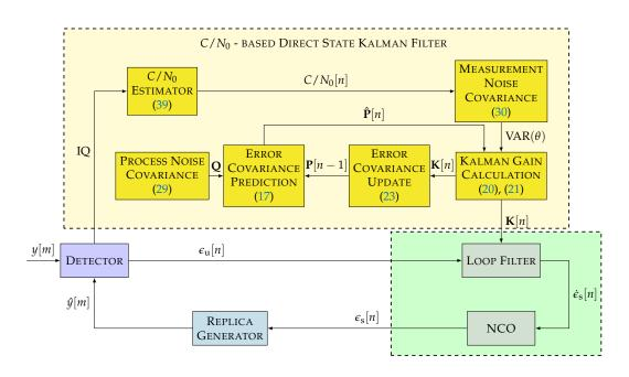
**Figure 8.** Non-linear model of the carrier-to-noise density ratio  $(C/N_0)$ -based DSKF.
