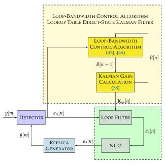
Figure 10. Non-linear model of LBCA-based LUT-DSKF.
