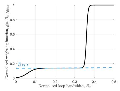
Figure 12. Selected Normalized weighting function in LBCA-based techniques.
