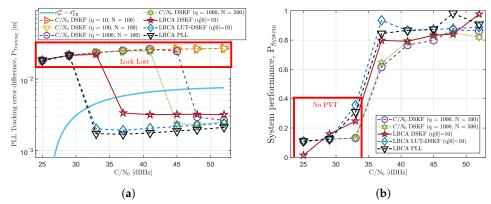
**Figure 15.** Dynamic performance of adaptive tracking techniques in third-order Costas PLL at different  $C/N_0$  levels. (a) Tracking performance of SV G17. (b) System performance.
