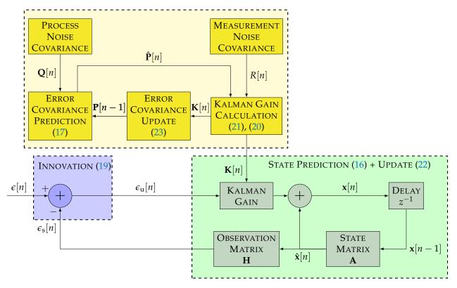
**Figure 4.** Linear model of the direct-state Kalman filter (DSKF) with m = 1. ©IEEE. Adapted, with permission, from [20].
