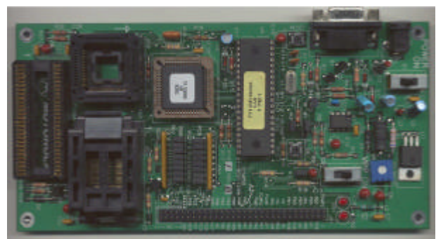
Figure 2. Motorola's in-circuit simulator kit
