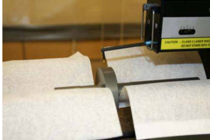
Figure 2.—Profilometry of Aeroflex Test Shaft.
