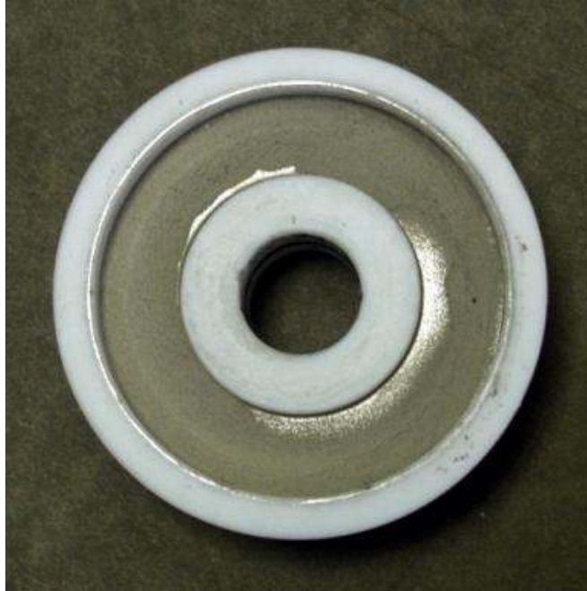
Figure 26.—NU-LHT-2M simulant found (~1.8 g) at base of Teflon cup after ~650,000 cycles testing in vacuum.
