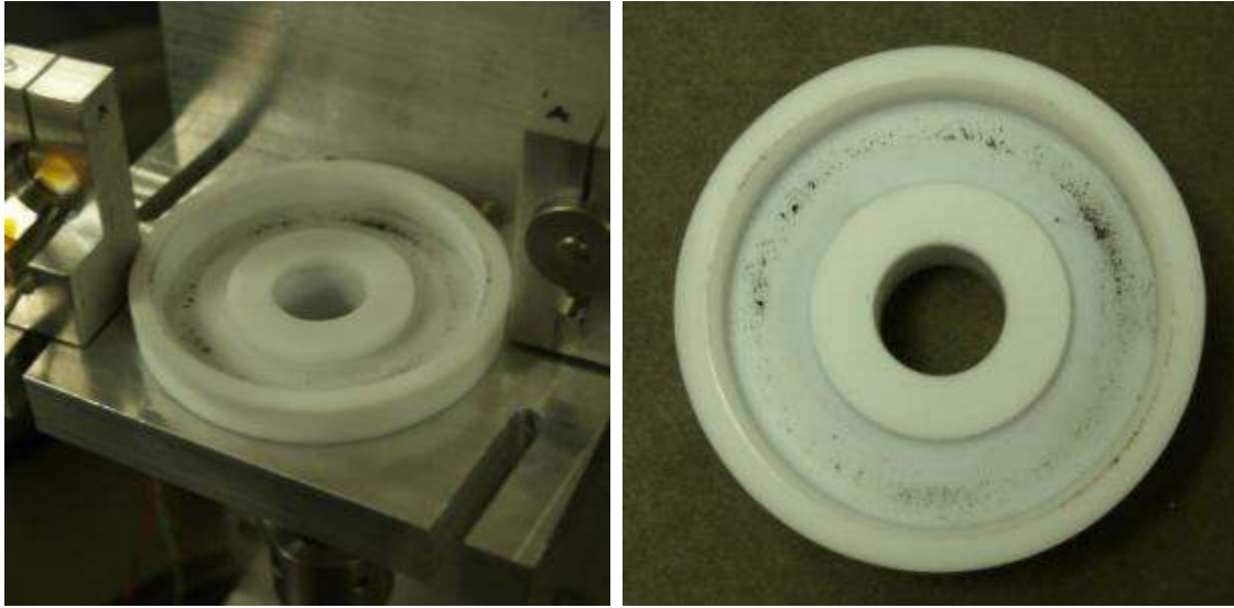
Figure 23.—NU-LHT-2M simulant found (~0.4 mg) at base of Teflon cup after 511,000 cycles in vacuum.
