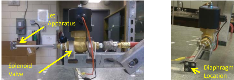
Fig. 6 Side view (left) and front view (right) of unsteady jet release apparatus.
