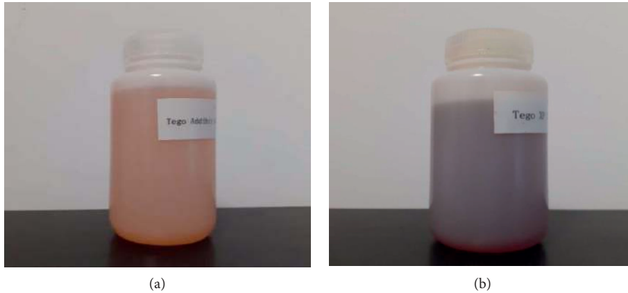
FIGURE 1: Silicone warm mix additives (a) Tego Addibit and (b) Tego XP.
