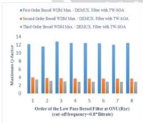
Fig-3:- Comparative analysis for various order of Bessel filter
