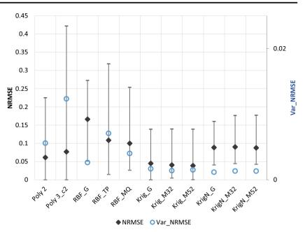
Therefore, Kriging modelling technique with Matérn 5/2 correlation function is shown to be the best method in terms of both accuracy and robustness over all types of problems for small sampling sizes.
