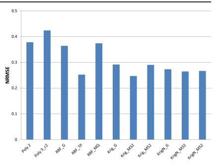
This result is consistent with the guideline provided which would have suggested the Kriging model with Matérn 3/2 correlation function—given the presence of noise.
