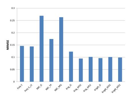
Fig. 20 NRMSE for the diesel engine NOx
