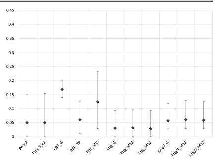
perform as well as Kriging models. It is also noted that for small and medium-scale problems Kriging with Gaussian correlation function performs particularly well. Of the RBF models, the RBFs with Thinplate kernel appear to perform best.
