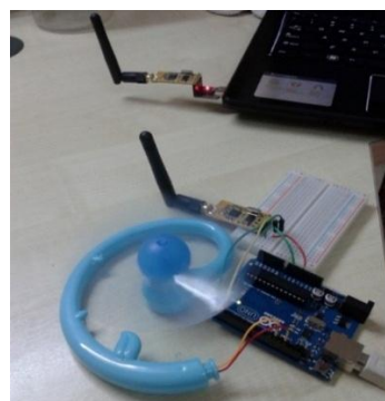
Figure 8. Experiment using APC220 Wireless Module
