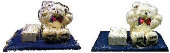
Fig. 12. Snapshot of the 3D reconstruction of Tea_and_bear scene obtained from: a) Kinect v1 data; b) Kinect v2 data.
