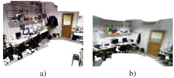
Fig. 13. Snapshot of the 3D reconstruction of a research laboratory obtained from: a) Kinect v1 data; b) Kinect v2 data.
