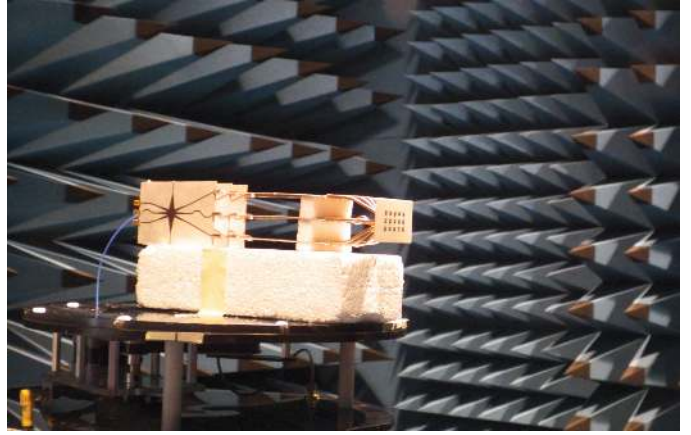
Fig. 3. Measurement setup in NSI anechoic chamber (photograph taken before covering the beamformer with absorbers).
