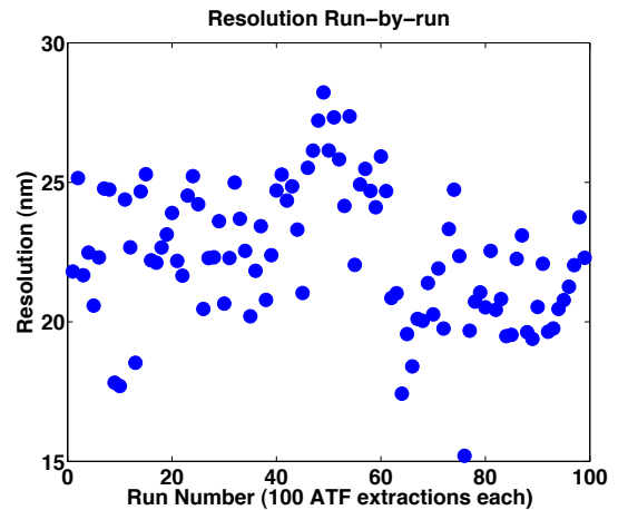
Fig. 24. Resolution for groups of (nominally) 100 sequential bunch crossings from 27 May 2005, 12:15 JST. The analysis employed the DDC algorithm with quality cuts. The mean resolution was 22.4 \pm 2.4 nm.
