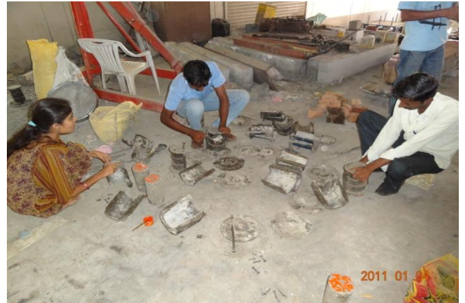
Fig. 6 Demoulding of GPC specimens
