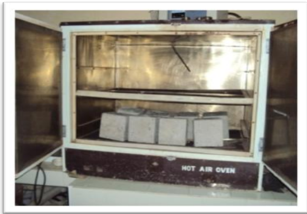
Fig. 3: Curing of GPC specimens
