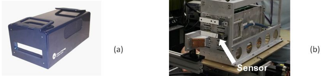
Figure 3. Two LPD detector prototypes are shown. (a) LPD 2-Tile detector prototype with 32 \times 256 pixels, and (b) LPD supermodule detector prototype partly populated with sensor tiles resulting in a 256 \times 256 pixels geometry.
