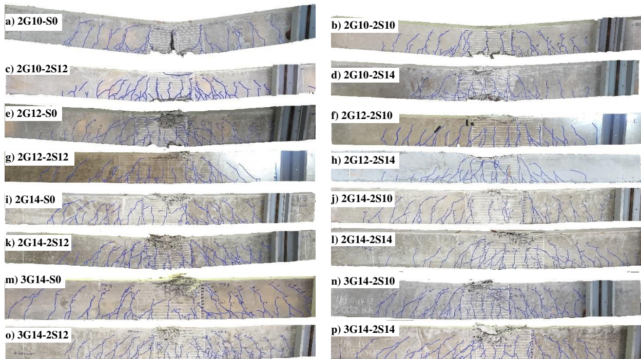
Figure 6. Crack patterns and failure modes of tested beams
