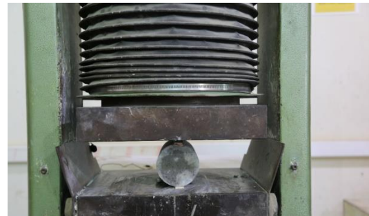
Fig.6: Specimen under splitting tensile test
