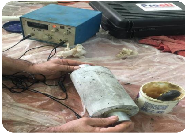
Fig.7: Pulse velocity of the concrete specimens.
