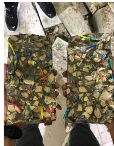
Fig.12: Fiber distribution after testing for PS-0.5 sample
