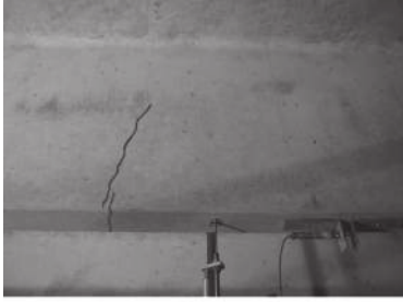
a) Initial Crack Propagation
