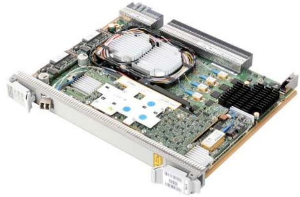
Fig. 7. Photograph of commercial 46 Gb/s DP-QPSK coherent transceiver.
