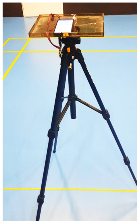
Figure 2. Stand used for manual data collection, consisting of a tripod and a mobile terminal on which an application for collecting measurement data is installed.
