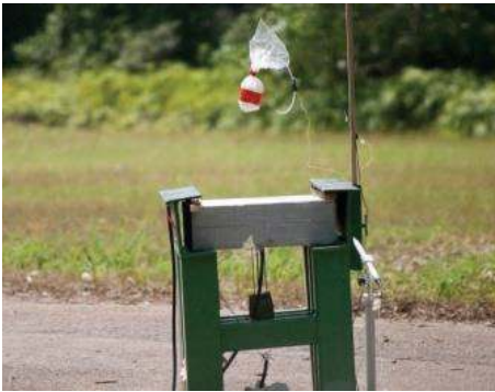
FIGURE 2: Field blast test setup.
