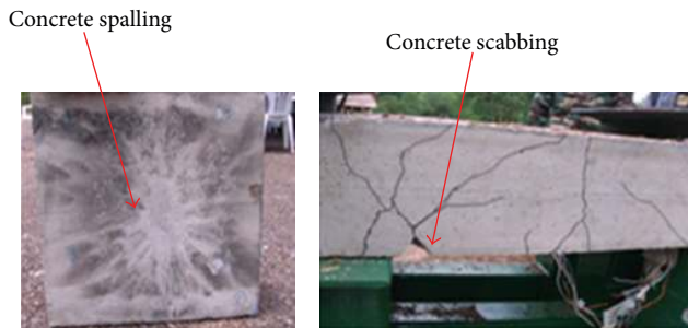
FIGURE 7: Failure mode of NRC panel subjected to blast loading.
