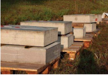
FIGURE 1: Reinforced concrete test panels.
