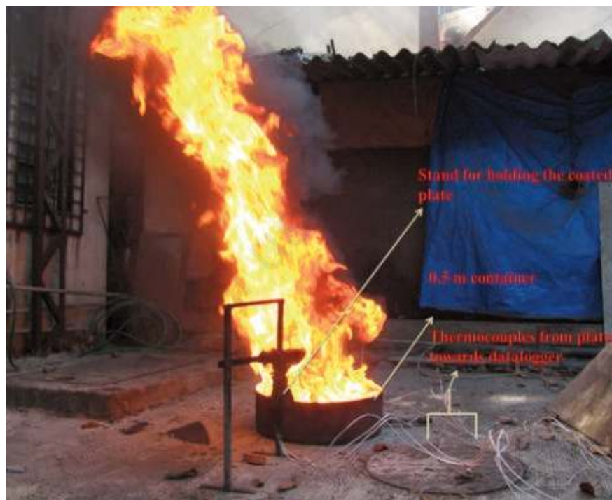
Figure 4. Photograph of the 0.5 m open pool diesel fire.
