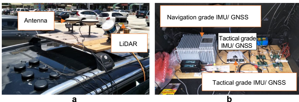
Fig. 6 Sensors Installation. a Top view of the vehicle; b Interior view of the vehicle
