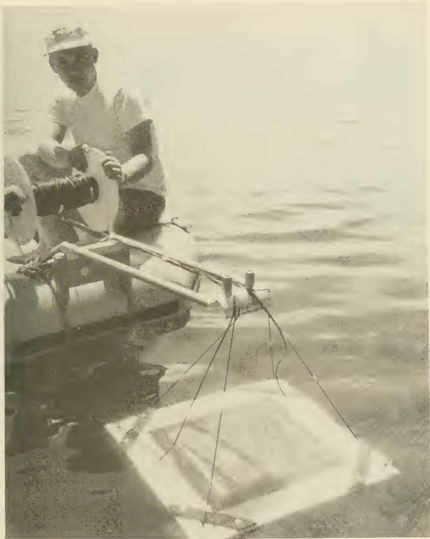
Figure 11. Deployment of solar cell panels from a surface raft by means of a hand-operated winch. Note that the two identical solar cell panels are mounted back-to-back in the wooden frame; the upward-facing panel measures downwelling irradiance, while the downward-facing panel measures the upwelling irradiance.
