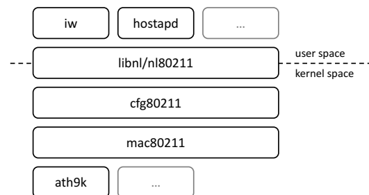
Figure 2. IEEE 802.11 Linux kernel implementation architecture. The support for 802.11p has to be present on all layers. [6]
