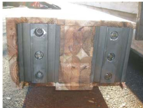
(a) Partial tensile failure of connection between LSB and plate in beam
