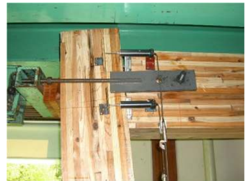
(b) Pullout failure of LSB in column
