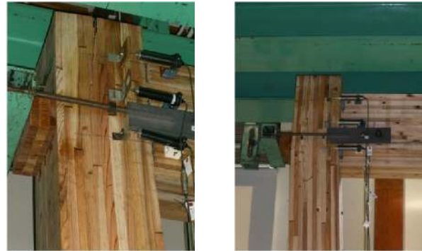
(a) Spilt at the top column (b) Bending crack on the column
