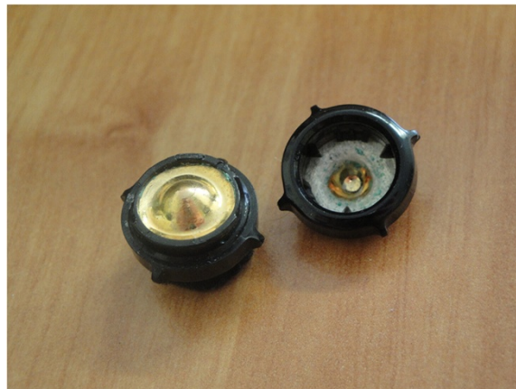
Figure 9 Oxidation of the electrodes. The oxidation of the electrode is clearly visible in green. On the back, the non-oxidized electrode has a gold color.
