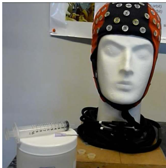
Figure 1 ANT device. The cables and the electrodes are well fixed in order to decrease motion artefacts. The cables are shielded to avoid interference.
