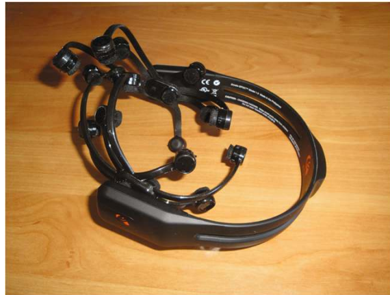
Figure 3 Emotiv picture. The Emotiv Epoc headset is handy to place and wireless.
