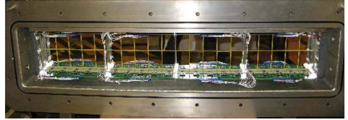
Figure 6. A picture of the Si wall (backside) showing the 40 Si detectors, preamplifiers and detector housing.
