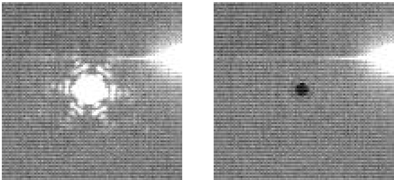
Figure 14. A latent image of a “star” found during the engineering instrument testing. The saturating point source image is shown on the left. The latent appears to affect only the offset of the starting signal level of the integration as shown in the right hand image—the measured affect on the slope is very small, less than a few electrons per second.
