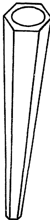
Fig. 14. Full-length view of (U,Zr)C (carbide) fuel element. Length, 0.64 m; across flats, 5.5 mm; coolant-channel diameter, 3.2 mm; and carbon/metal atom ratio, 0.8 to 0.92.
