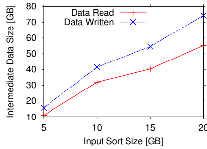
(b) TeraSort Total Amount of Data Read and Written. The amount of intermediate data generated that is being written and read is significantly greater than the original sort size. This intermediate data degrades CVM's performance the most in TeraSort.
