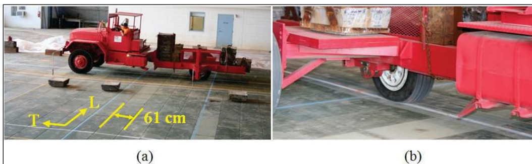
Figure 2. Aircraft simulator (a) Overall view of test section and (b) Close-up view of load wheel.
