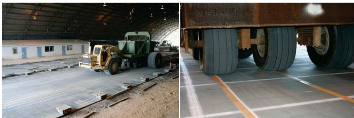
Figure 20. AM2 matting panels trafficked by C-17 aircraft simulator in full-scale test section.
