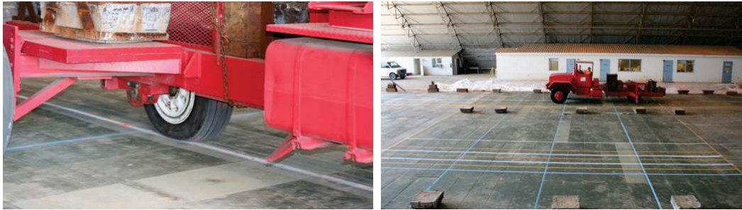
Figure 9. AM2 matting panels trafficked by aircraft simulator in full-scale test section.
