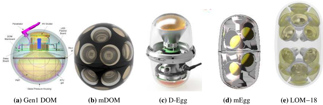
Figure 1: Schematic view of the optical modules. Gen-1 DOMs are used for the IceCube array, and mDOM and D-Eggs will be deployed in the IceCube-Upgrade holes. mEgg and LOM-18 are two designs for IceCube Gen2 studied here.
