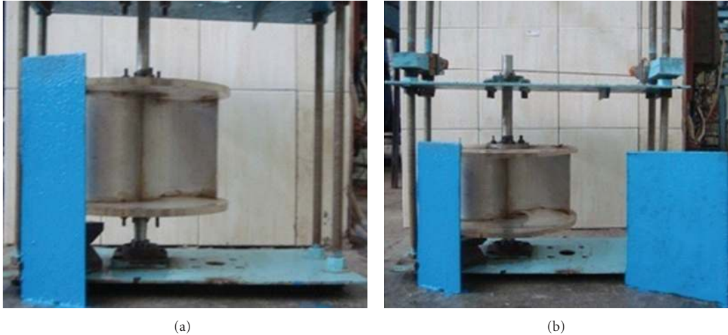
FIGURE 14: Pictorial representation of the modified Savonius rotor with deflector plate on the returning blade side (a) and rotor with two deflector plates (b).
